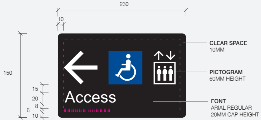
TYPICAL GRAPHIC SETOUT 01: ACCESSIBLE ACCESS (Scale 1:4)
