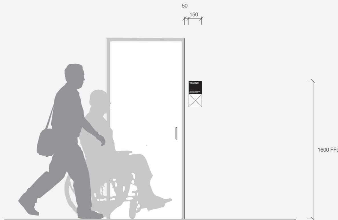
TYPICAL FRONT ELEVATION: CO LOCATED WITH S.38 ROOM SIGN SUPPLEMENTARY PANEL (Scale 1:25)
