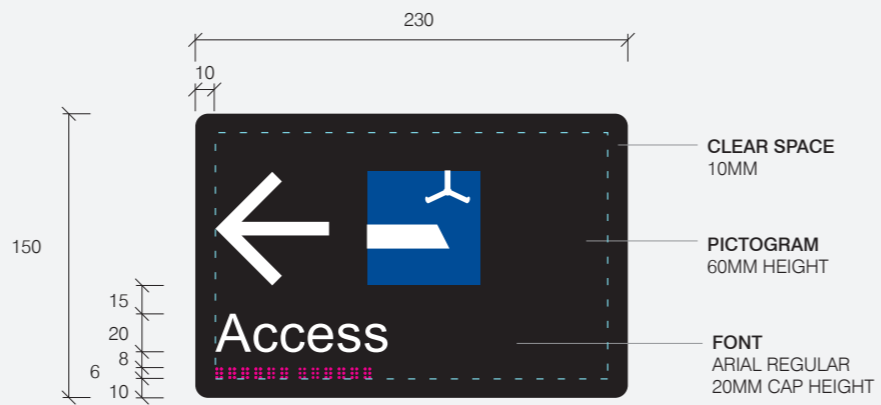
TYPICAL GRAPHIC SETOUT 06: ACCESSIBLE ACCESS - CHANGING (Scale 1:4)
