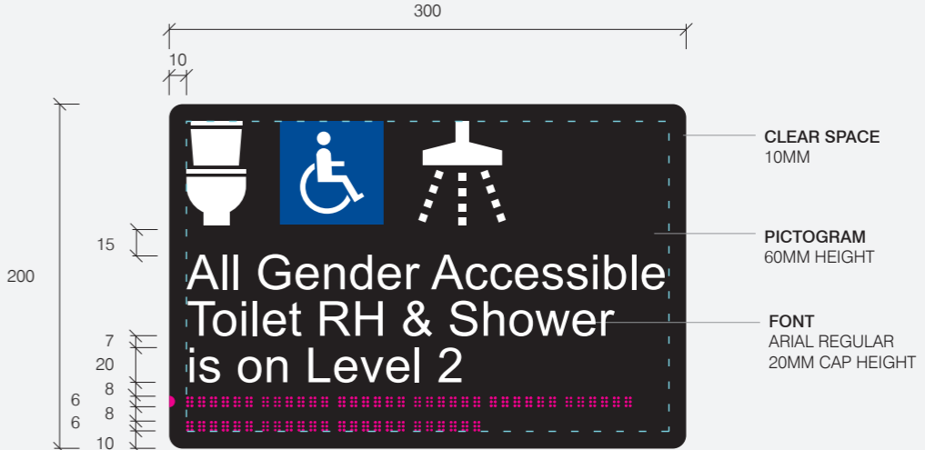
TYPICAL GRAPHIC SETOUT 04: ACCESSIBLE ACCESS - AMENITIES (Scale 1:4)
