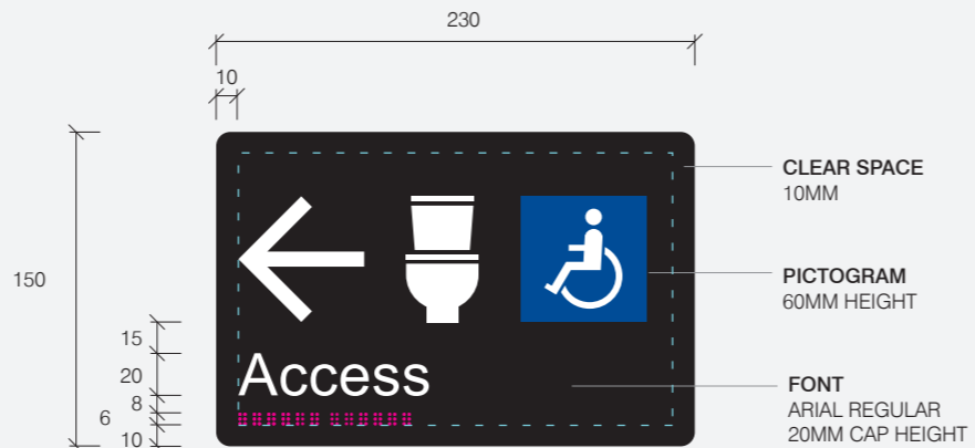
TYPICAL GRAPHIC SETOUT 03: ACCESSIBLE ACCESS - AMENITIES (Scale 1:4)
