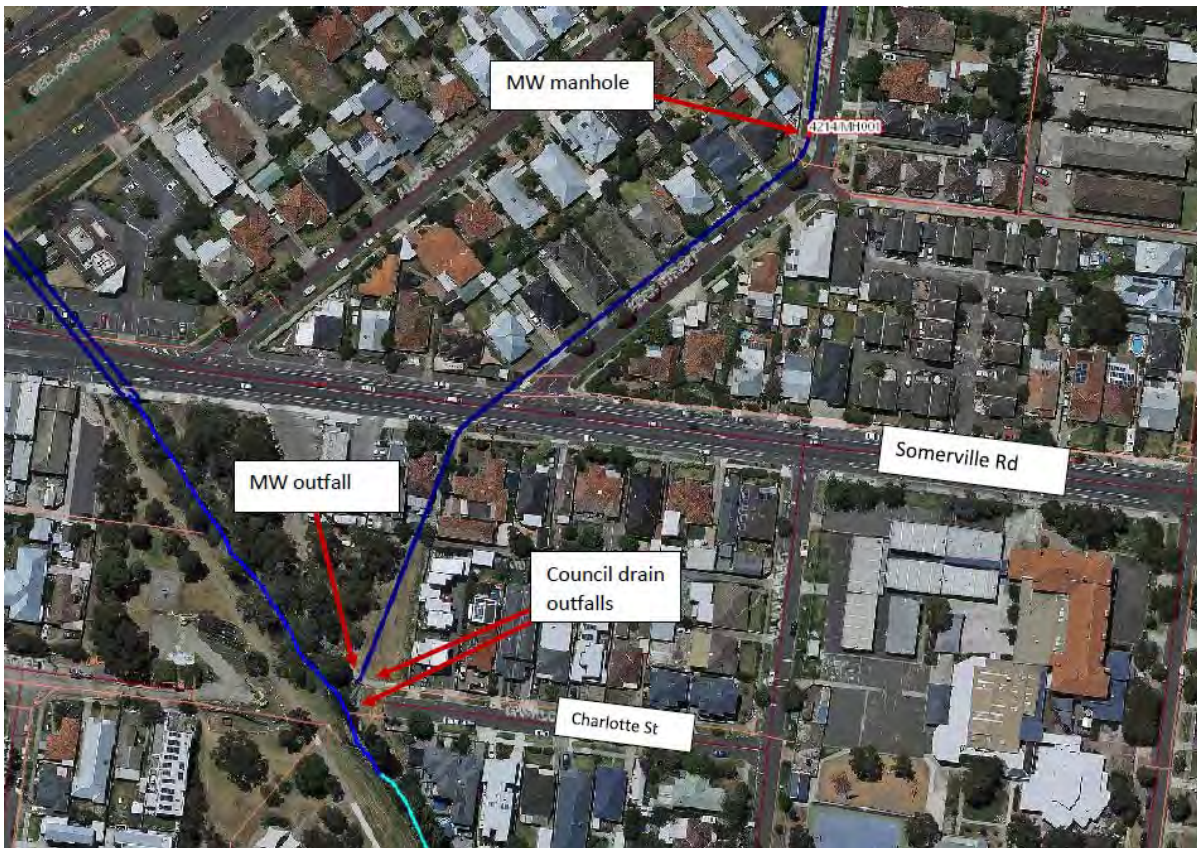
Figure 12 Location of manholes and drain outfall at Charlotte St.
