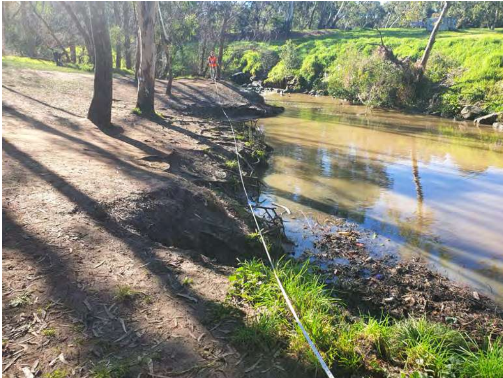
Figure 4. Unevenly eroded bank. Line of best fit used. Note: Zone A falls on the steep slope. Only sample sections you can access safely.
