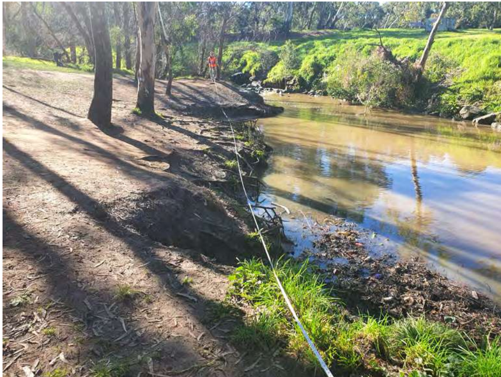
Figure 4. Unevenly eroded bank. Line of best fit used. Note: only sample sections you can access safely.
